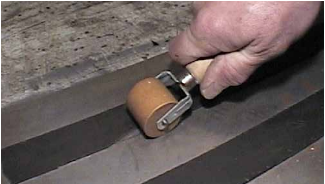
When you are satisfied with the arrangement of the Damper Pads or Strips, pressure roll them to the metal surface with a wallpaper seam roller, as illustrated.
